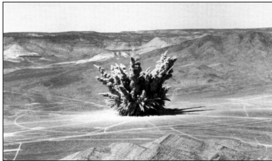
This 1955 test of an 8000 lb. nuclear bomb buried 67 feet deep had a 1.2 kiloton yield comparable to that of a low-yield "mini-nuke" earth penetrator. The Nevada Test Site blast, which was obviously not contained and would have produced grave "collateral damage," left a crater that was 300 feet wide and 128 feet deep.
